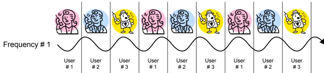
TDMA is used in communications networks such as the Global System for Mobile Communications (GSM), Integrated Digital Enhanced Network (iDEN, a technology that combines a mobile phone with a two-way dispatch business radio) and Personal Digital Cellular (PDC), a system used in Japan.
